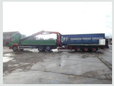
I.D. Number : C150117 Chassis Number : SMU DFC 27B3L0 30033 First Registered : 01.11.2003 20Ft 6ins Flatbed Body C/w Raised Headboard And Wood Plank Floor . BPW Axles C/w 385/65R 22.5 Tyres. Air Suspension C/w Raise And Lower Controls. Full Drum Brake System C/w Haldex ABS System. Jost Landing Leg. Plated Weight : 24,000 Kgs. Design Weight : 27,000 Kgs. Tested Until End : October 2020. Vehicle Length: 17.5 Mtrs. Vehicle Height: 3.7 Mtrs.
