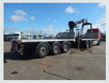
Entwisle Tri Axle Chassis. 18Ft óins Flatbed Body C/w Raised Headboard And Aluminium Flooring. Mercedes Axles Axles C/w 385 65R 22.5 Wheels And Tyres. Full Disc Braking System. Air Suspension. Haldex ABS/EBS C/w Iso Susie Connector. Dual Speed Landing Leg. Plated Weight : 21,000 Kgs. Design Weight : 21,000 Kgs. Tested Until End : Expired. Total Height : 3.6 Mtrs. Total Width : 2.5 Mtrs. Total Length : 16.8 Mtrs.
