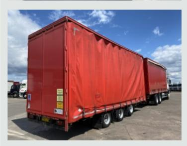
Rear Aperture : 9Ft 11ins. Side Aperture : 9Ft 11ins. Internal Height : 10Ft 3ins.
