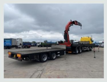
SM Tandem Axle Chassis. 19Ft Flatbed Body C/w Raised Headboard, Wood Plank Flooring And Lashing Rings. Mercedes Axles C/w 245 70R 19.5 Wheels And Tyres. Air Suspension C/w Raise And Lower Controls. Haldex ABS/EBS Disc Brake System. Dual Speed Landing Legs. O/s And N/s Chassis Mounted Storage Lockers. Plated Weight : 18,000 Kgs. Design Weight : 18,000 Kgs. Tested Until End : Expired. Total Height : 3.9 Mtrs. Total Width : 2.5 Mtrs. Total Length : 18.7 Mtrs. Spec Number: 29194
