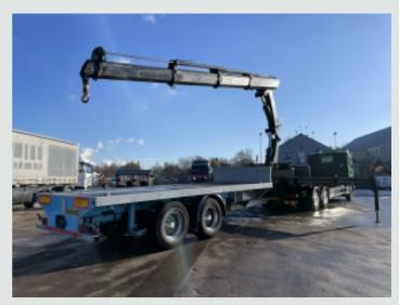
22Ft Flatbed Body C/w Raised Headboard, Wood Plank Flooring, Lashing Rings And 4x Twistlocks.
