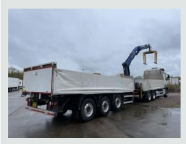
Air Suspension. Disc Braking System. Alcoa Alloy Wheels.
