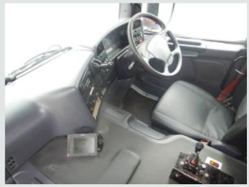
Air Suspension C/w Raise And Lower Controls.
