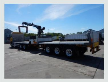
Chassis No: 080057 First Reg : 01.05.2008 Cartwright Tri Axle Chassis. 19Ft 5ins Flatbed Body C/w Raised Headboard And Aluminium Flooring. ROR Drum Axles Axles C/w 385 65R 22.5 Wheels And Tyres. Full Drum Braking System. Air Suspension C/w Raise and Lower. Front Lift Axle. Haldex ABS/EBS C/w Iso Susie Connector. Dual Speed Landing Leg. Plated Weight : 24,000 Kgs. Design Weight : 24,750 Kgs. Tested Until End : May 2018. Total Height : 3.6 Mtrs. Total Width : 2.5 Mtrs. Total Length : 18.2 Mtrs.
